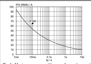
Fig.4. Maximum non-repetitive rms forward current.  $I_F = f(t_p)$ ; sinusoidal current waveform;  $T_j = 150^{\circ}\text{C}$  prior to surge with reapplied  $V_{\text{RWM}}$ .
