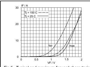
Fig.5. Typical and maximum forward characteristic;  $I_F = f(V_F)$ ; parameter  $T_j$
