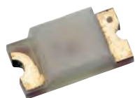
CHIPLED Bauform 1206 · CHIPLED Type 1206
