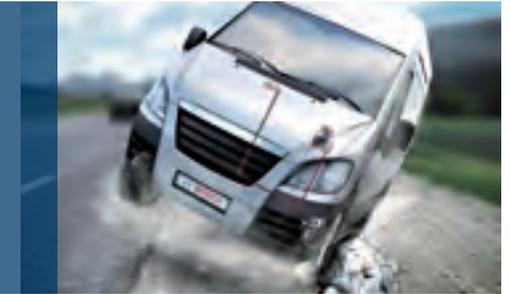
In case of an accident, a rollover situation can be securely detected with these MEMS angular rate sensors. The sensors are available with either analog or digital output. Angular rate sensors for rollover detection.
