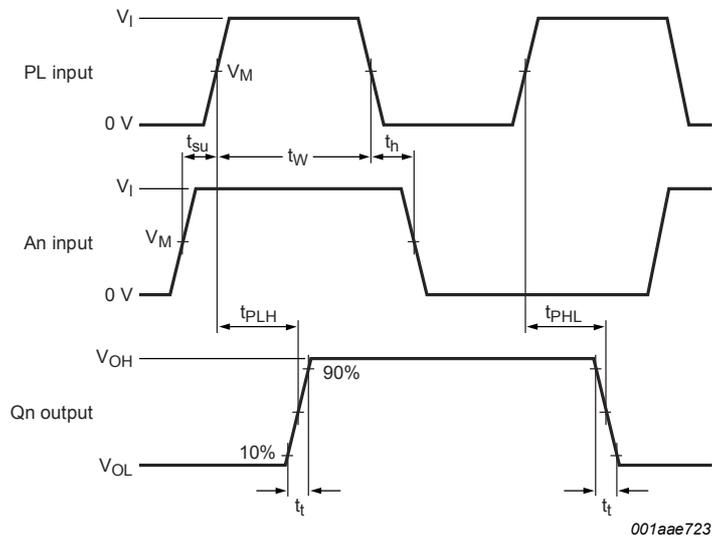
b. Propagation delays for PL and An to Qn, setup and hold times for PL to An, Qn transition times and minimum PL pulse width
