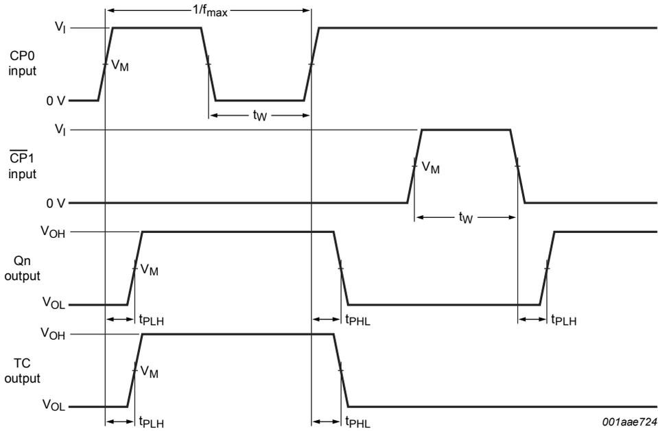
a. Propagation delays for CP0,  $\overline{CP1}$  to Qn, and TC, minimum CP0 and  $\overline{CP1}$  pulse widths and maximum frequency
