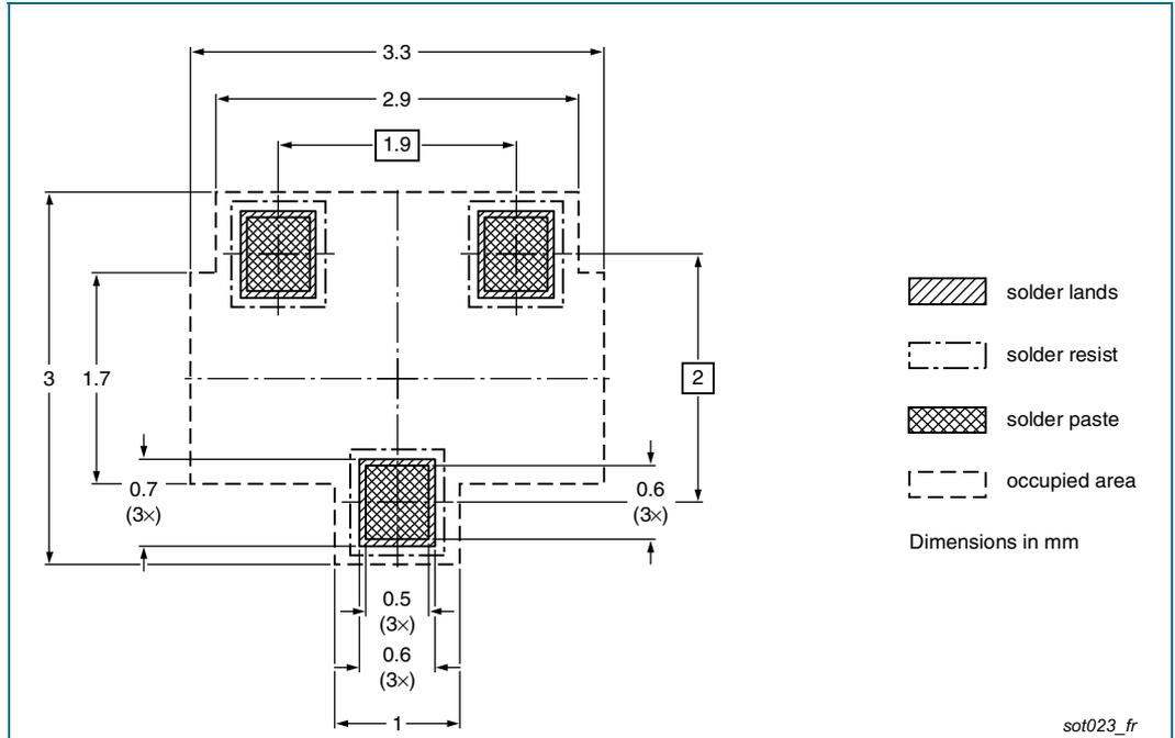
Fig 4. Reflow soldering footprint SOT23 (TO-236AB)
