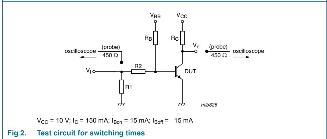
Fig 2. Test circuit for switching times
