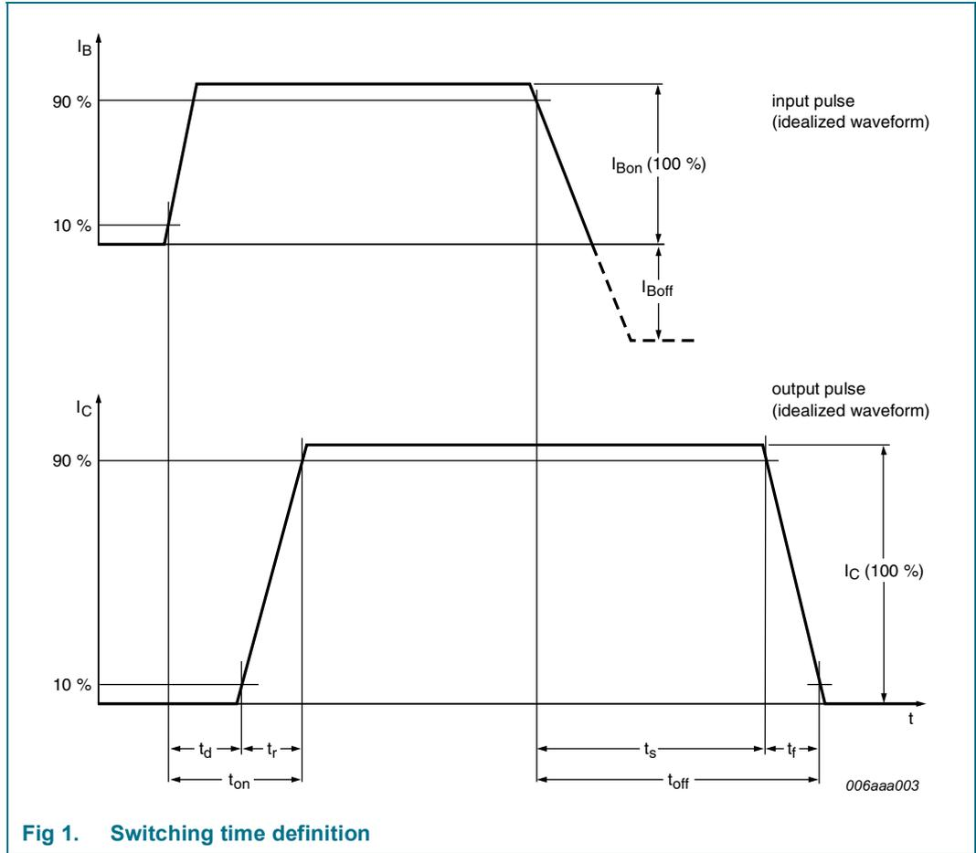
Fig 1. Switching time definition
