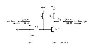
$$\begin{split} &V_i = -9.5 \text{ V}; \text{ T} = 500 \text{ }\mu\text{s}; \text{ } t_p = 10 \text{ }\mu\text{s}; \text{ } t_r = t_f \leq 3 \text{ ns}. \\ &\text{R1} = 68 \text{ }\Omega; \text{ R2} = 325 \text{ }\Omega; \text{ }R_B = 325 \text{ }\Omega; \text{ }R_C = 160 \text{ }\Omega. \\ &V_{BB} = 3.5 \text{ V}; \text{ }V_{CC} = -29.5 \text{ V}. \\ &\text{Oscilloscope: input impedance } Z_i = 50 \text{ }\Omega. \end{split}$$
