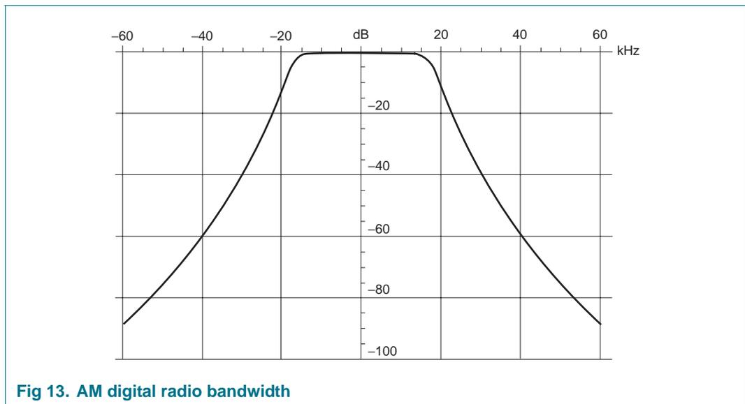
Fig 13. AM digital radio bandwidth
