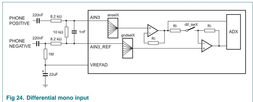
Fig 24. Differential mono input
