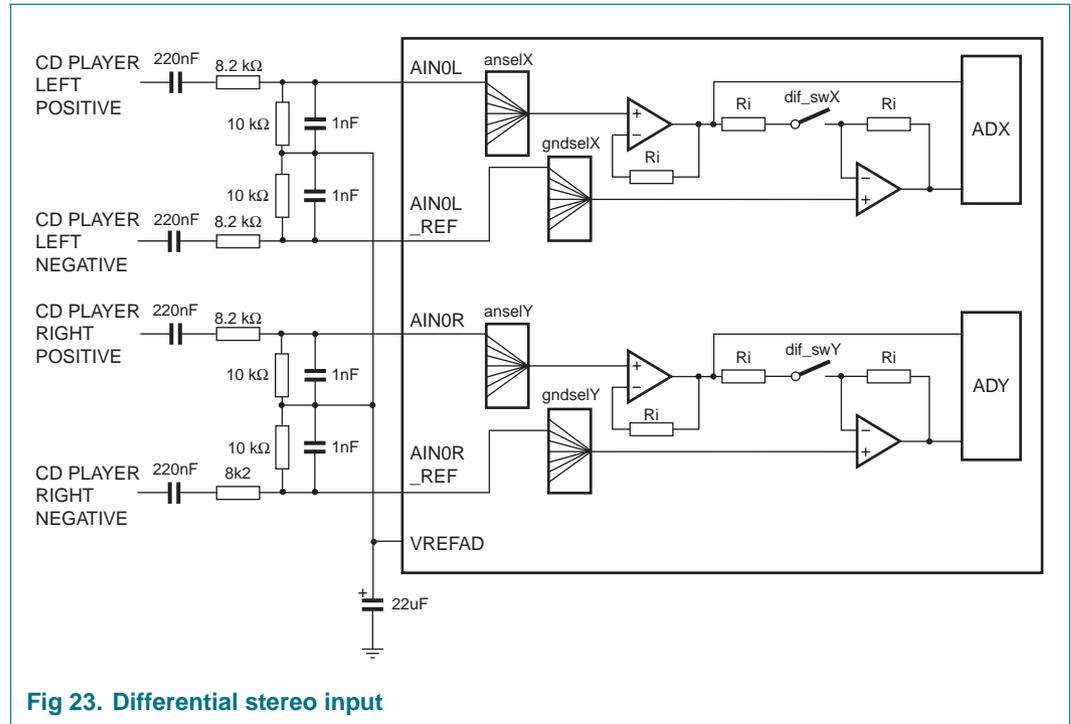
Fig 23. Differential stereo input
