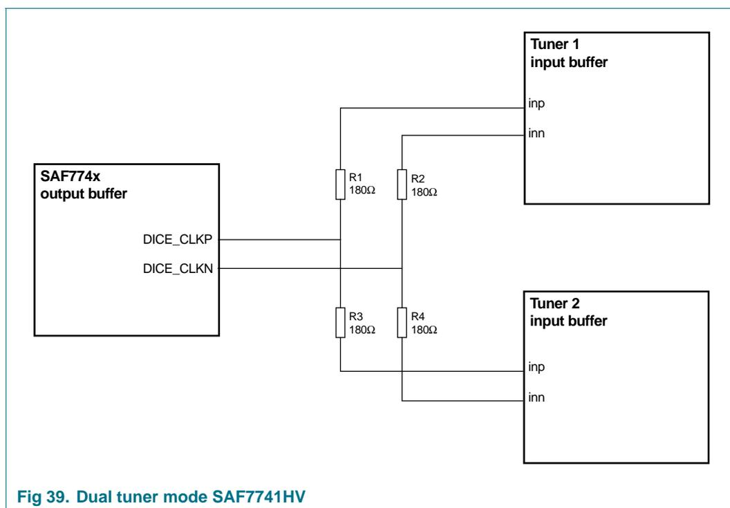
Fig 39. Dual tuner mode SAF7741HV
