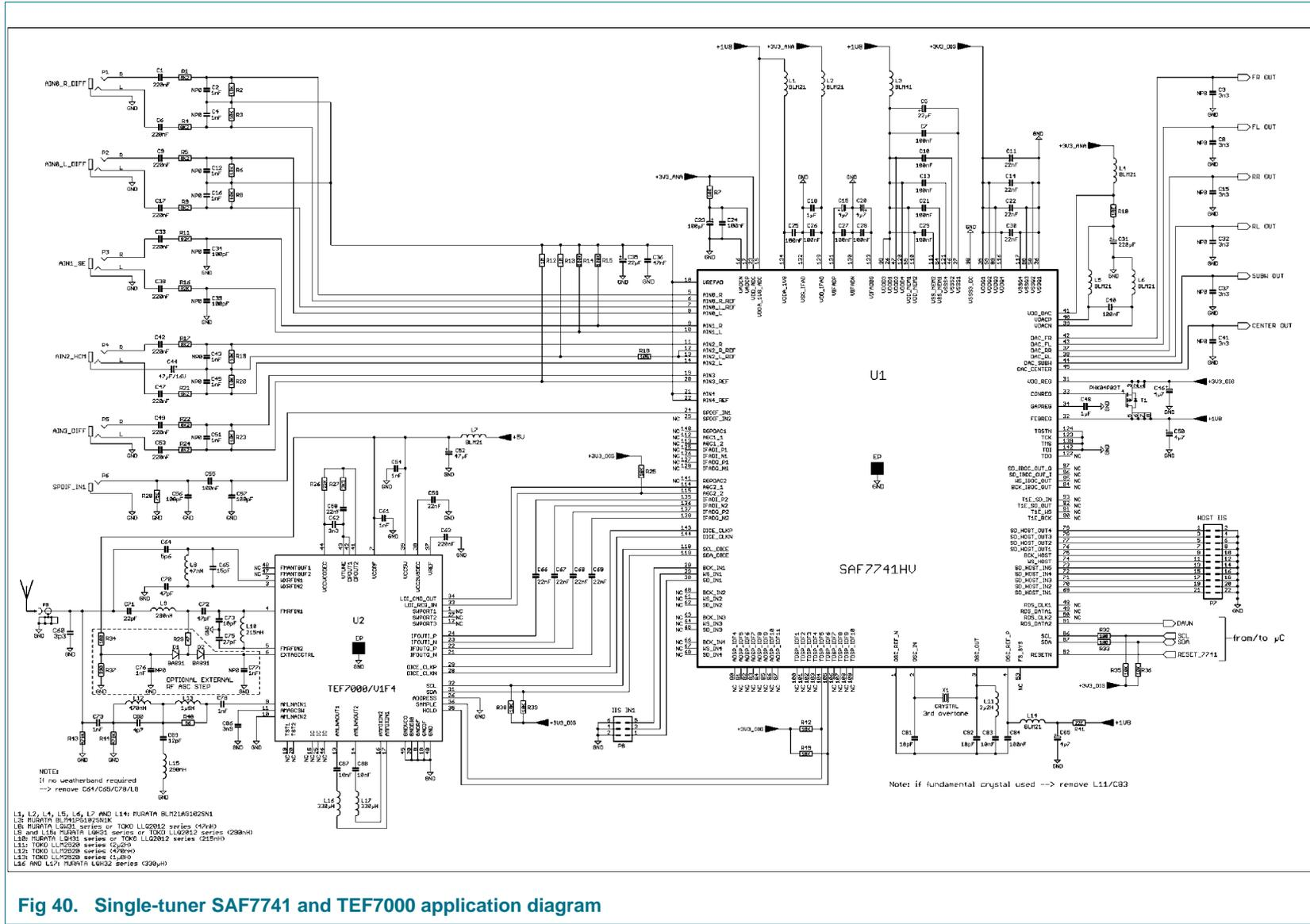
Fig 40. Single-tuner SAF7741 and TEF7000 application diagram
