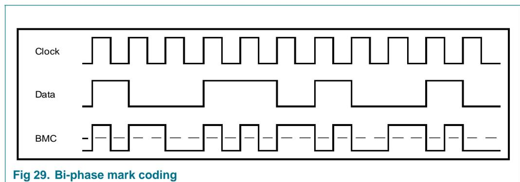
Fig 29. Bi-phase mark coding
