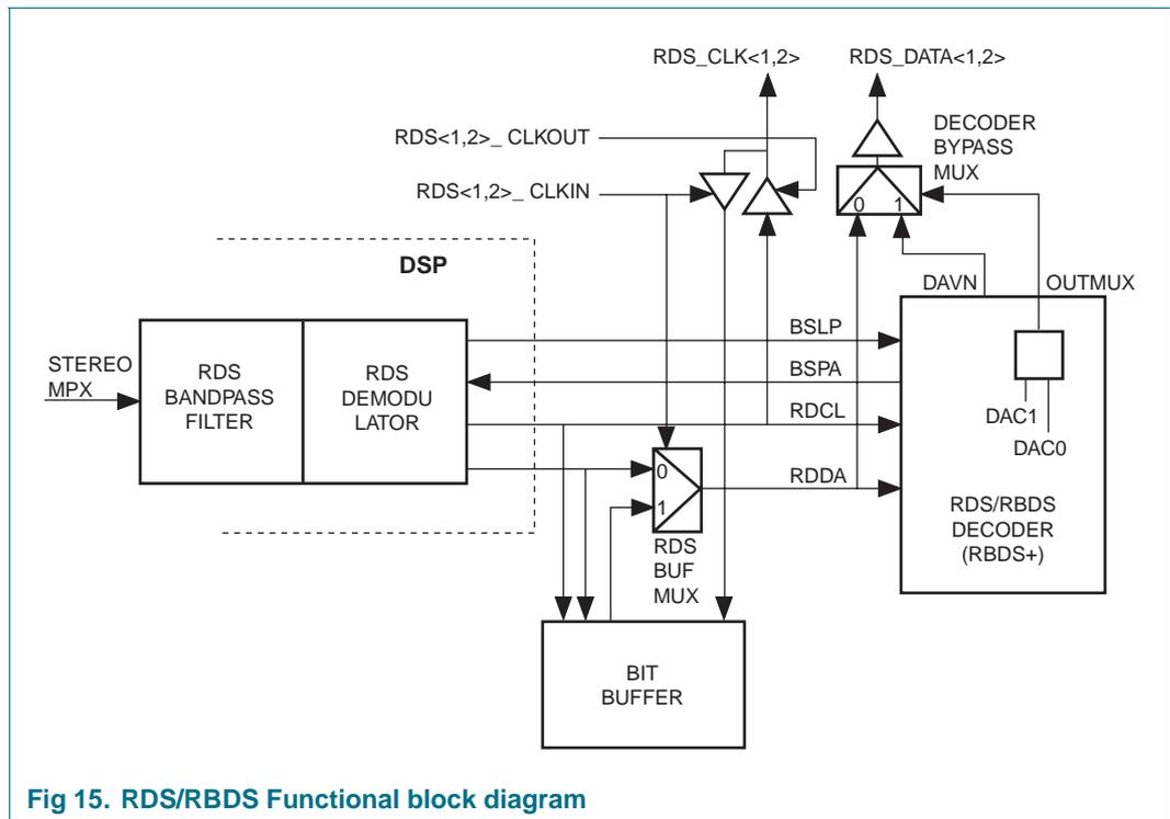
Fig 15. RDS/RBDS Functional block diagram
