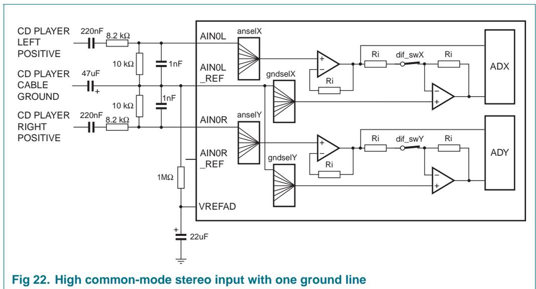
Fig 22. High common-mode stereo input with one ground line
