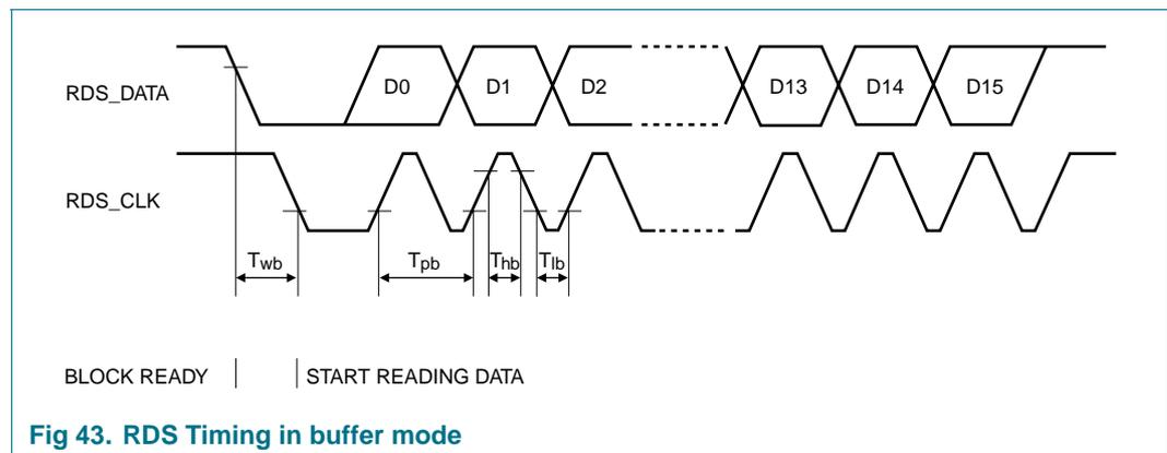
**Fig 43. RDS Timing in buffer mode**
