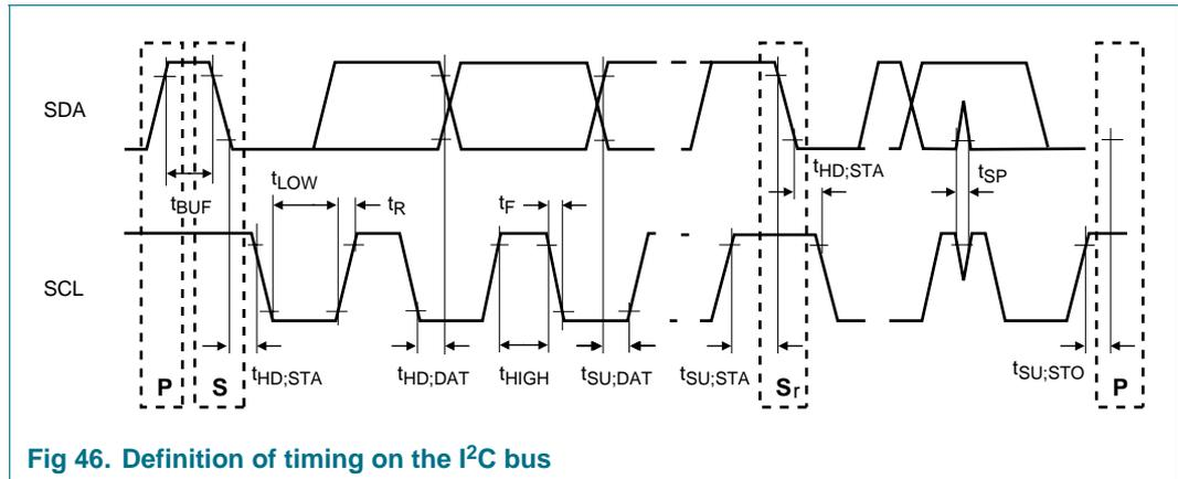
Fig 46. Definition of timing on the I<sup>2</sup>C bus
