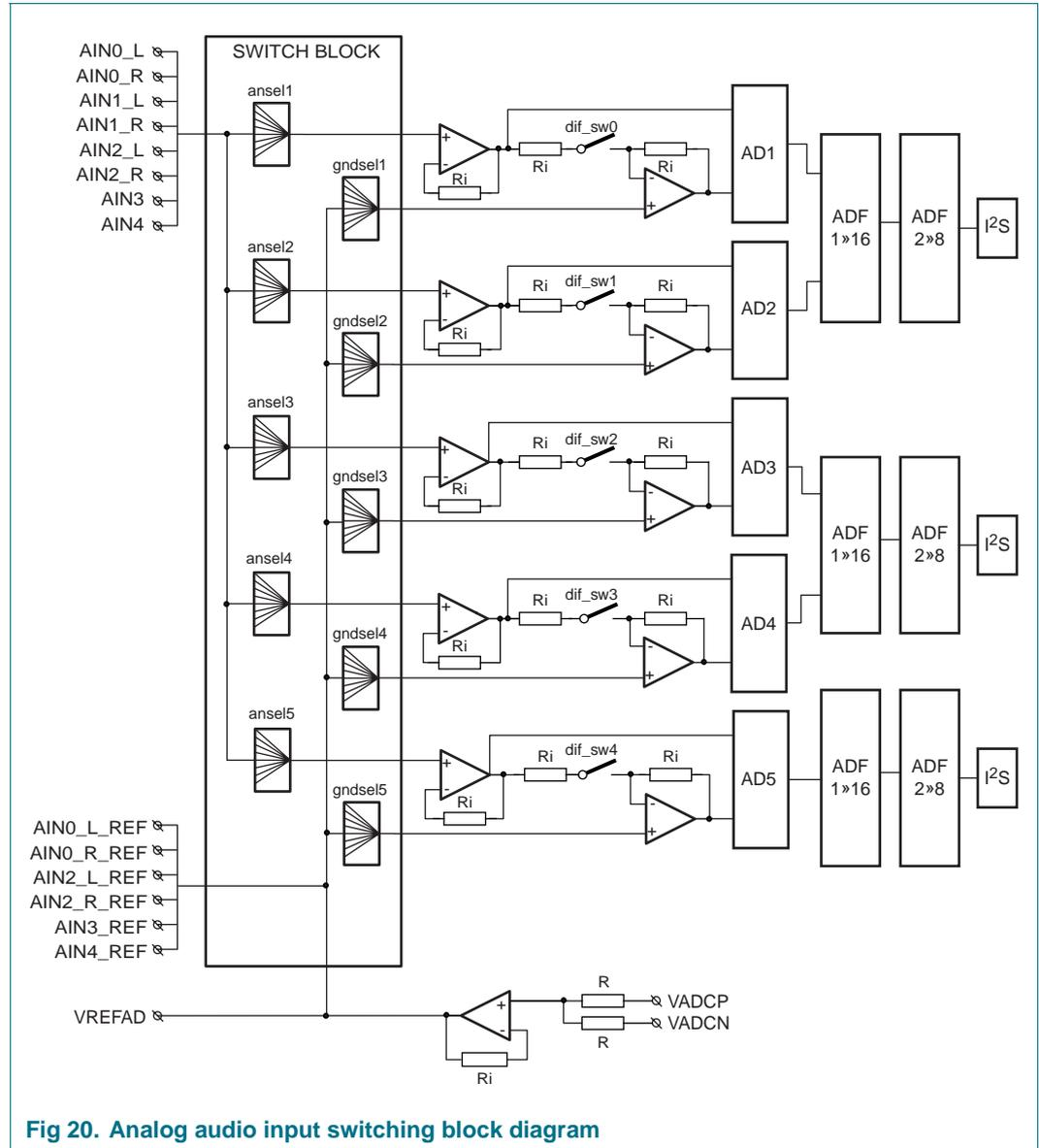
Fig 20. Analog audio input switching block diagram
