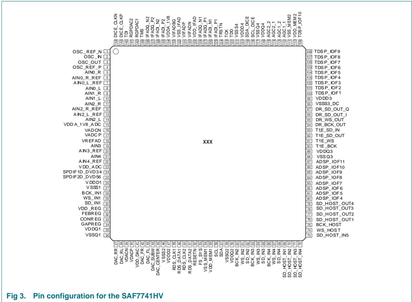
Fig 3. Pin configuration for the SAF7741HV
