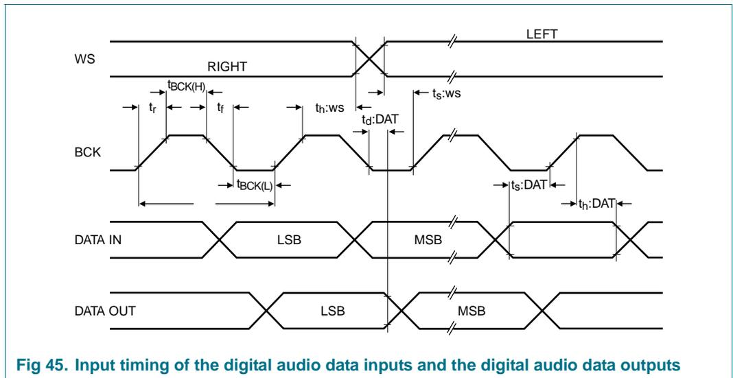
Fig 45. Input timing of the digital audio data inputs and the digital audio data outputs
