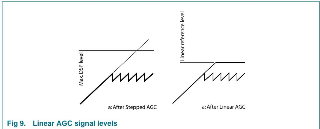
The linear control reference level should be above the maximum uncontrolled input level of the linear control stage (See [Figure 7](#)). Settings of the reference level below the maximum uncontrolled input level will result in a distorted output signal.
