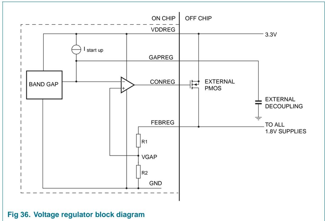
Fig 36. Voltage regulator block diagram
