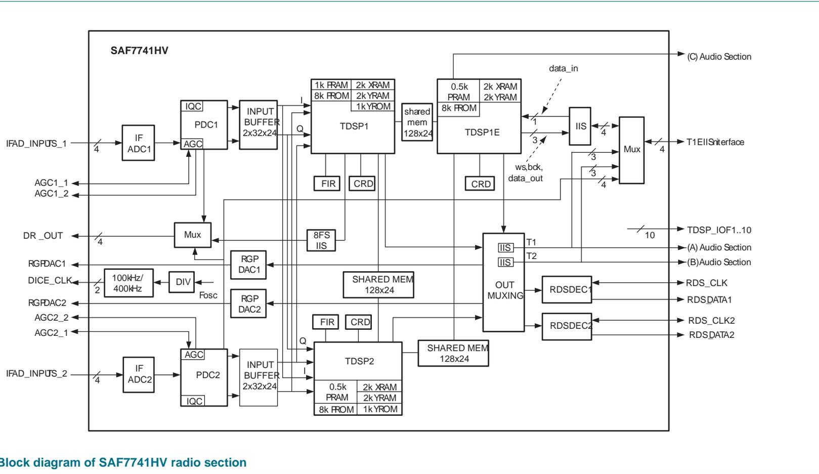
Fig 1. Block diagram of SAF7741HV radio section
