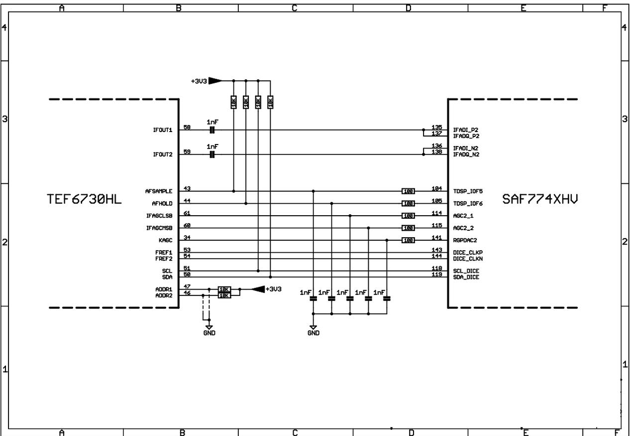
Fig 41. SAF774x and TEF6730 connections
