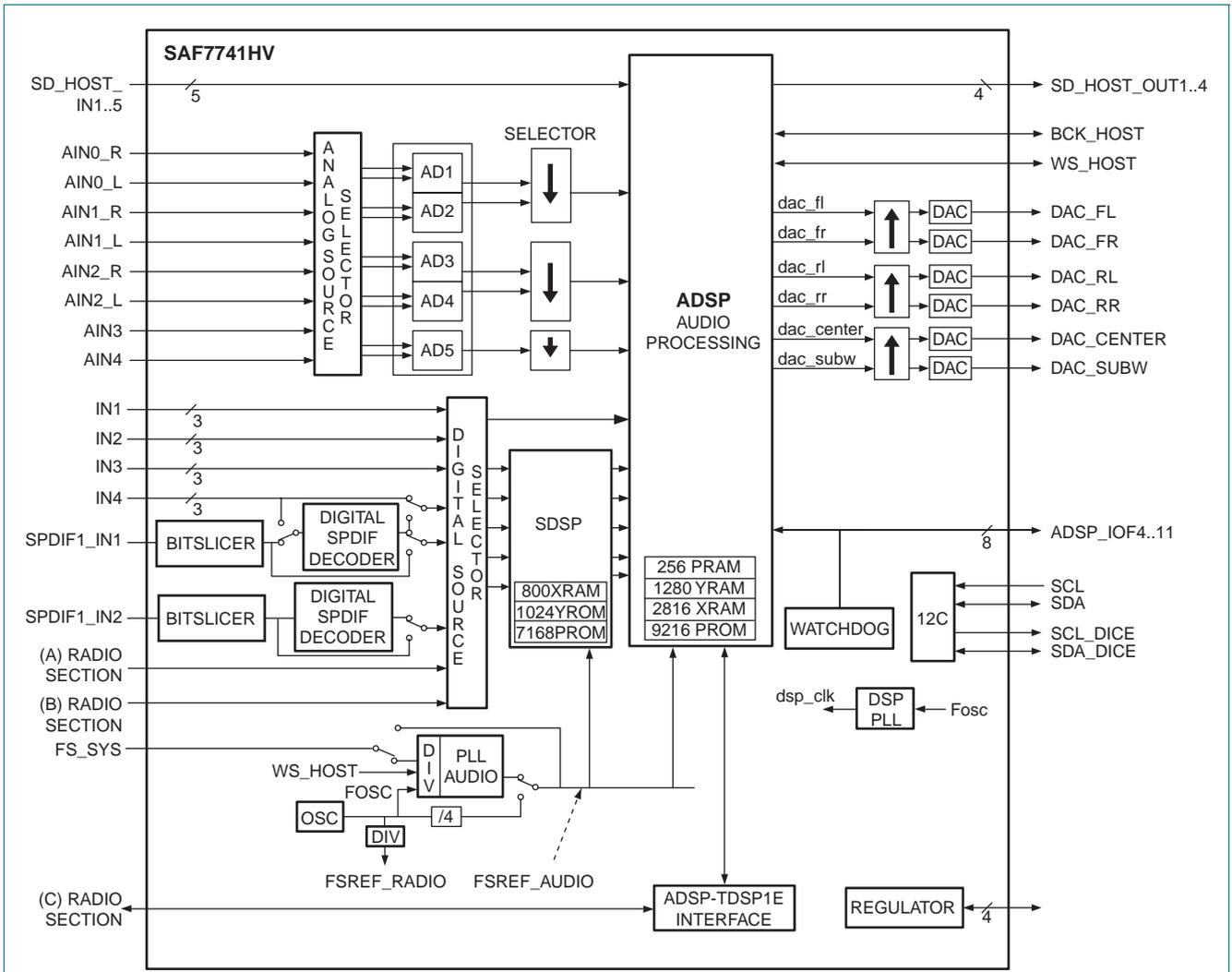
Fig 2. Block diagram of SAF7741HV audio section
