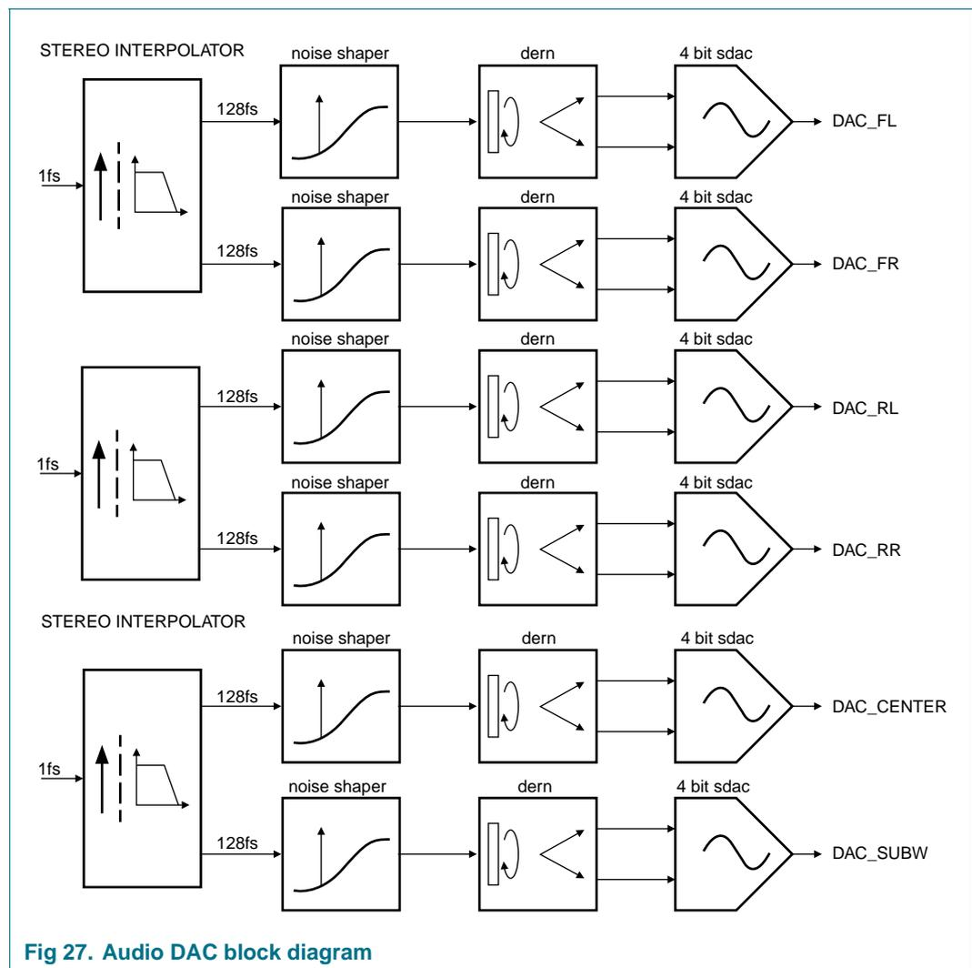
Fig 27. Audio DAC block diagram
