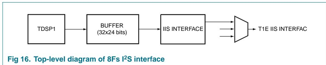
**Fig 16. Top-level diagram of 8Fs I<sup>2</sup>S interface**
