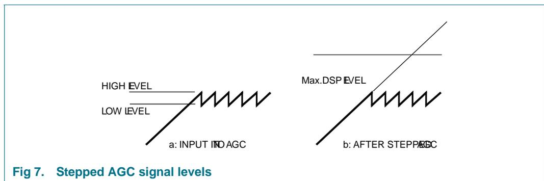
Fig 7. Stepped AGC signal levels
