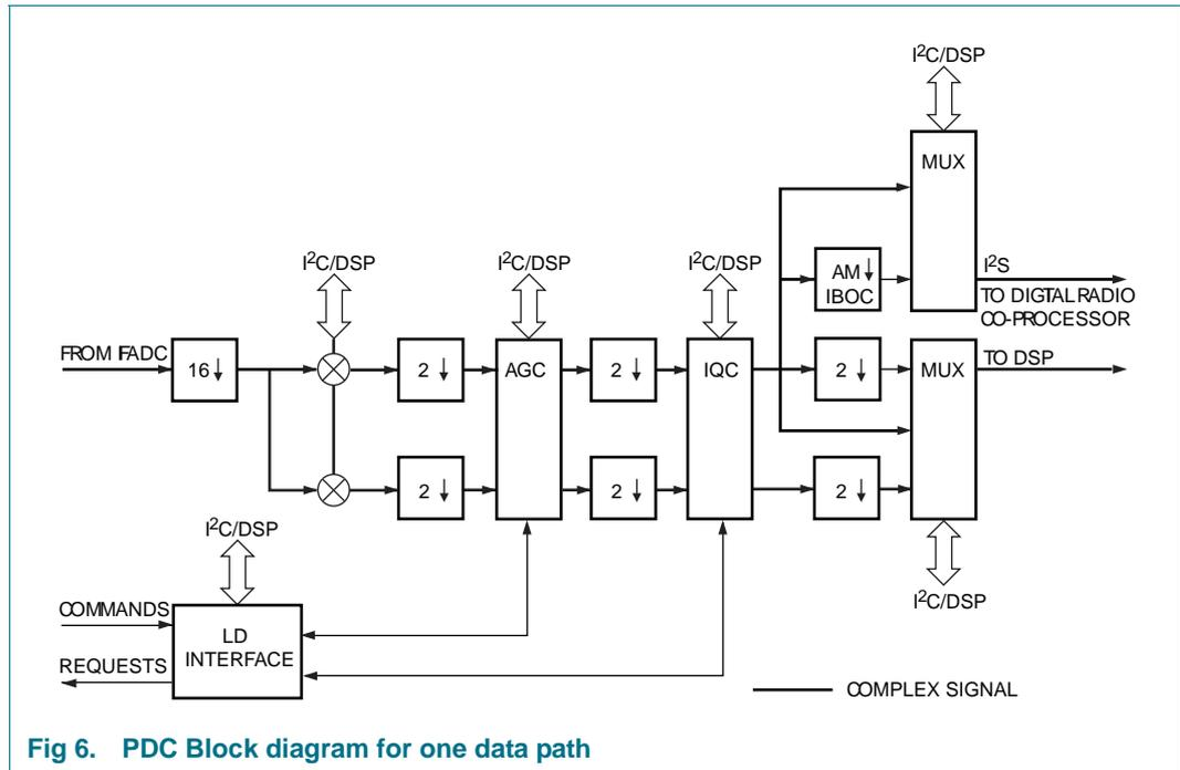
Fig 6. PDC Block diagram for one data path
