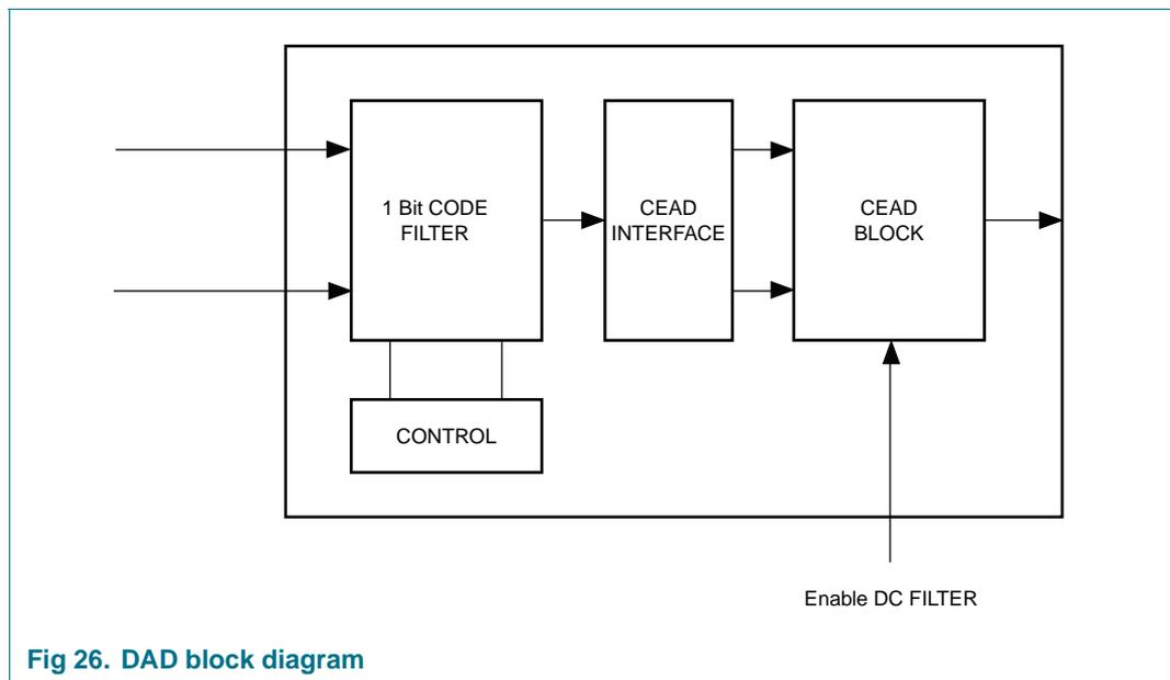
The input signal has a sample frequency of  $128 \times f_s$  and comes from a third-order  $\Sigma\Delta$  ADC. The first step in the decimation process is done by the 1-bit code Cascaded Integrator Comb (CIC) filter and Audio Decimation Filter 1 (ADF1) filter. See [Figure 26](#). The CIC filter decimates the input sample rate by a factor of 16 and thus results in a sample rate of  $8 \times f_s$ .
