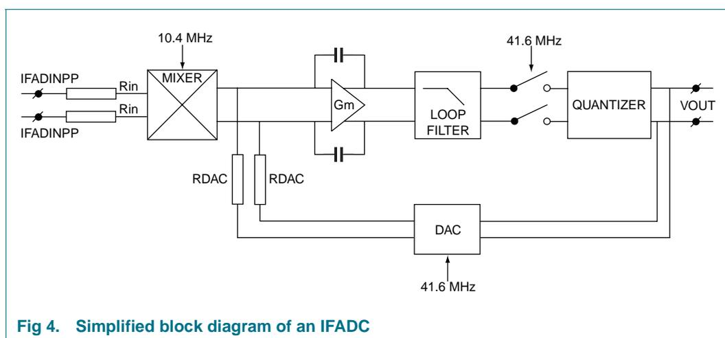
Fig 4. Simplified block diagram of an IFADC
