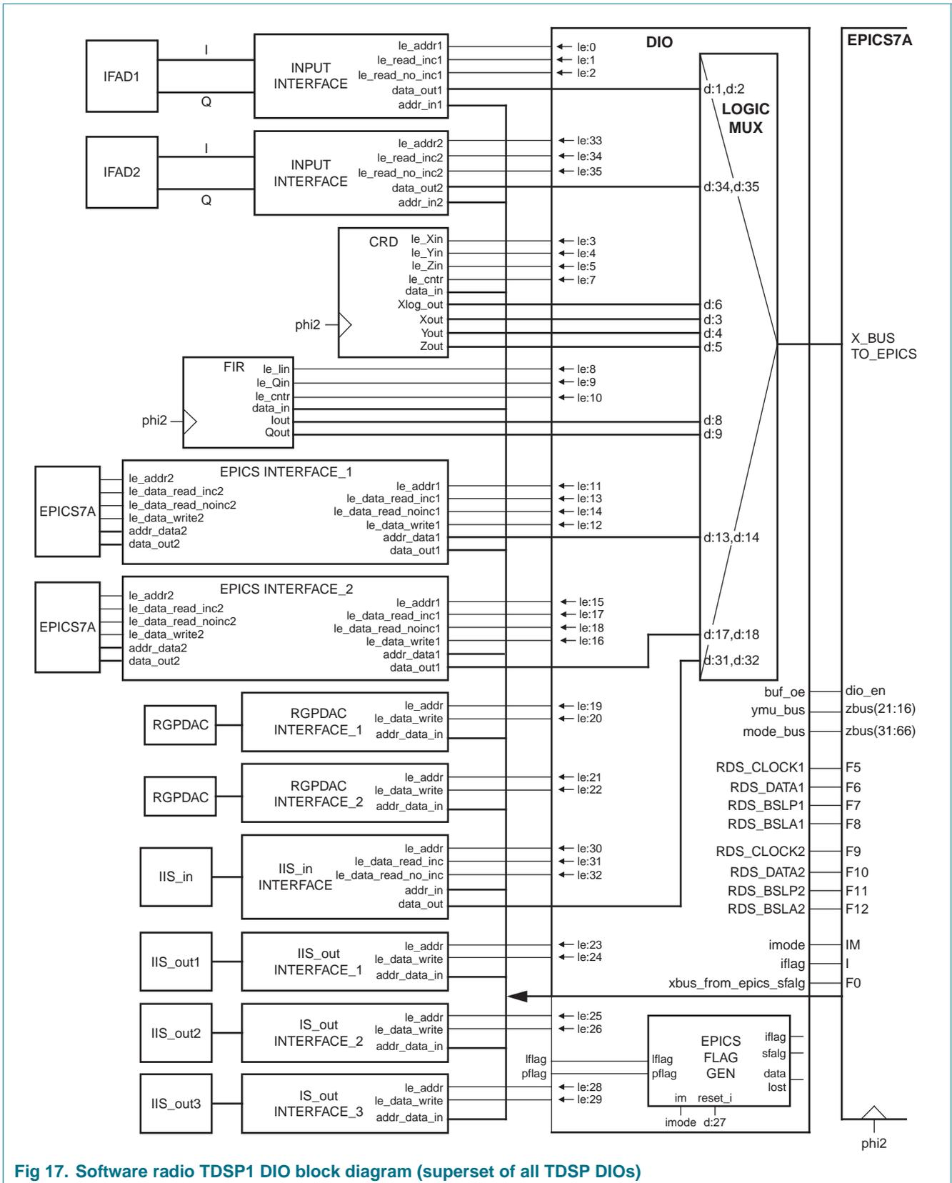
Fig 17. Software radio TDSP1 DIO block diagram (superset of all TDSP DIOs)
