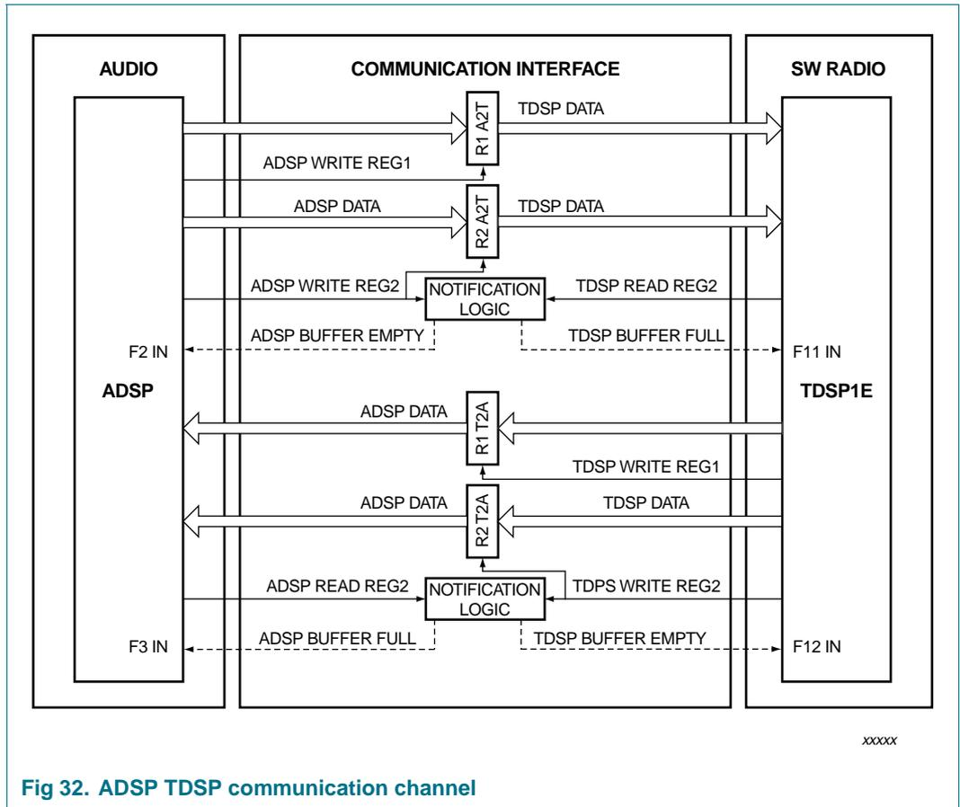
Fig 32. ADSP TDSP communication channel
