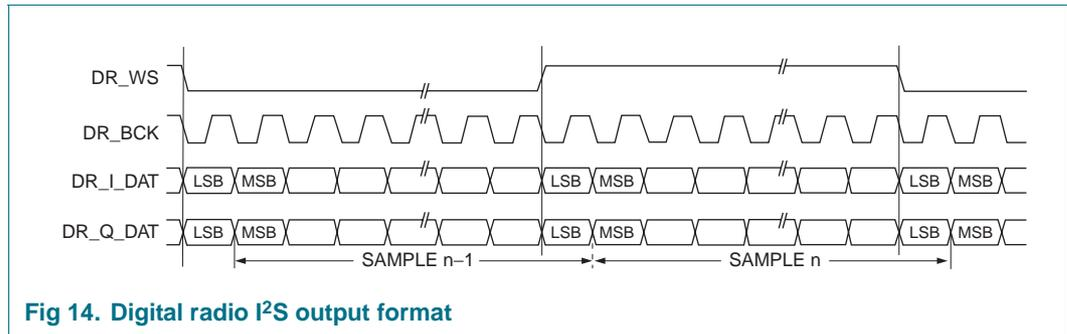
Fig 14. Digital radio I<sup>2</sup>S output format
