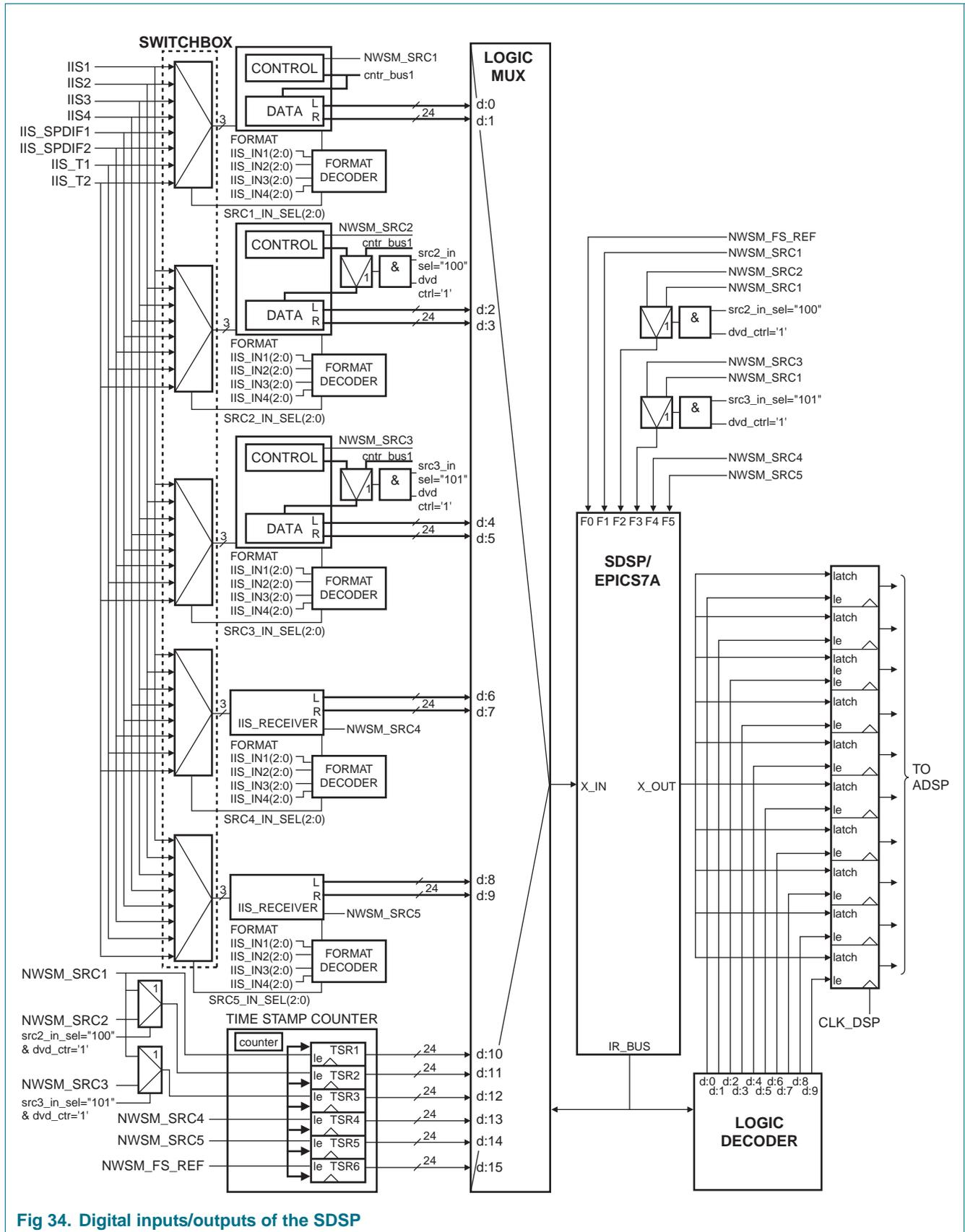
Fig 34. Digital inputs/outputs of the SDSP
