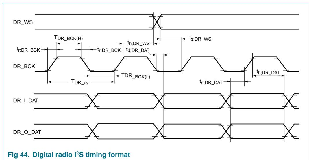
**Fig 44. Digital radio I<sup>2</sup>S timing format**
