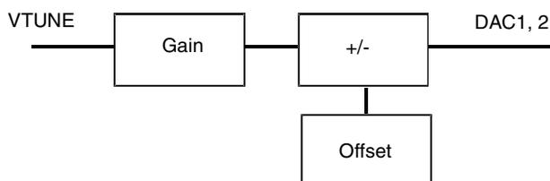
The gain of DAC1 and DAC2 has a range of approximately  $0.67 \times V(\text{VTUNE})$  to  $2.09 \times V(\text{TUNE})$ . This range is divided into 255 steps. One step is approximately  $(2.09 - 0.67)/255 = 0.00557 \times V(\text{TUNE})$ . The gain of DAC1 can be controlled by the Bits 38 to 45 ( $2^0$  to  $2^7$ ) and the gain of DAC2 can be controlled by the Bits 66 to Bit 73 ( $2^0$  to  $2^7$ ) as given in Table 28.
