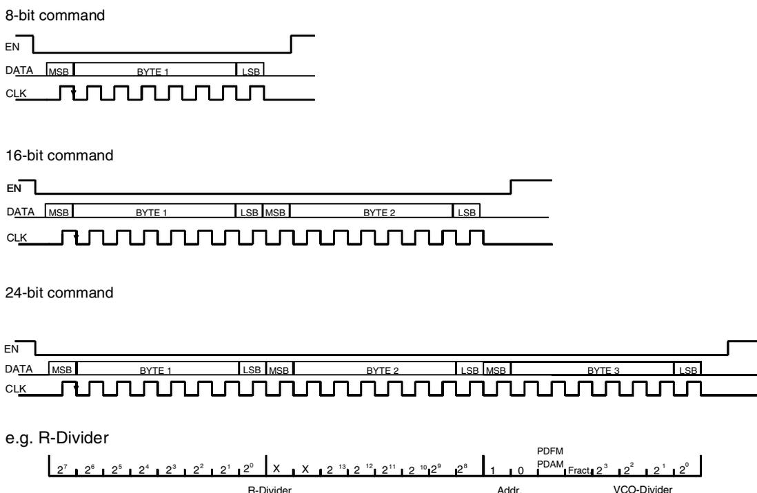
**Figure 4. 3-wire Bus Timing Diagram**
