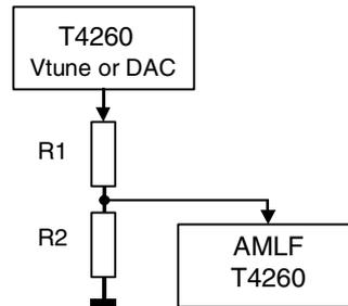
The maximum input voltage at the AMLF input (pin 17) depends on the applied supply voltage as well as on the gain and offset settings. To avoid any damages during the product's lifetime, the following formulas regarding SWAMLF voltage, gain and offset settings have to be observed (see also chapter Permitted DAC Conditions).
