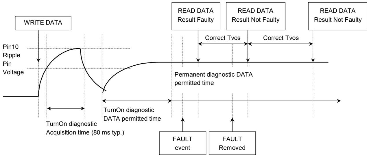
**Figure 8 Software Output Offset Detection Timing Chart**
