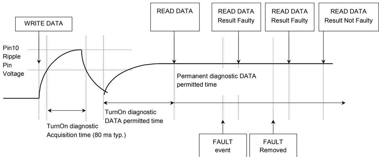
**Figure 7 Permanent Diagnosis Timing Chart for Each Short Detection**
