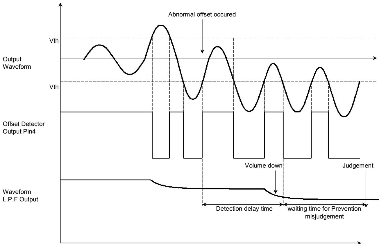
**Figure 9 Hardware Output Offset Detection**
