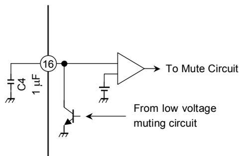
**Figure 2 Pin 16 Muting Circuit**
