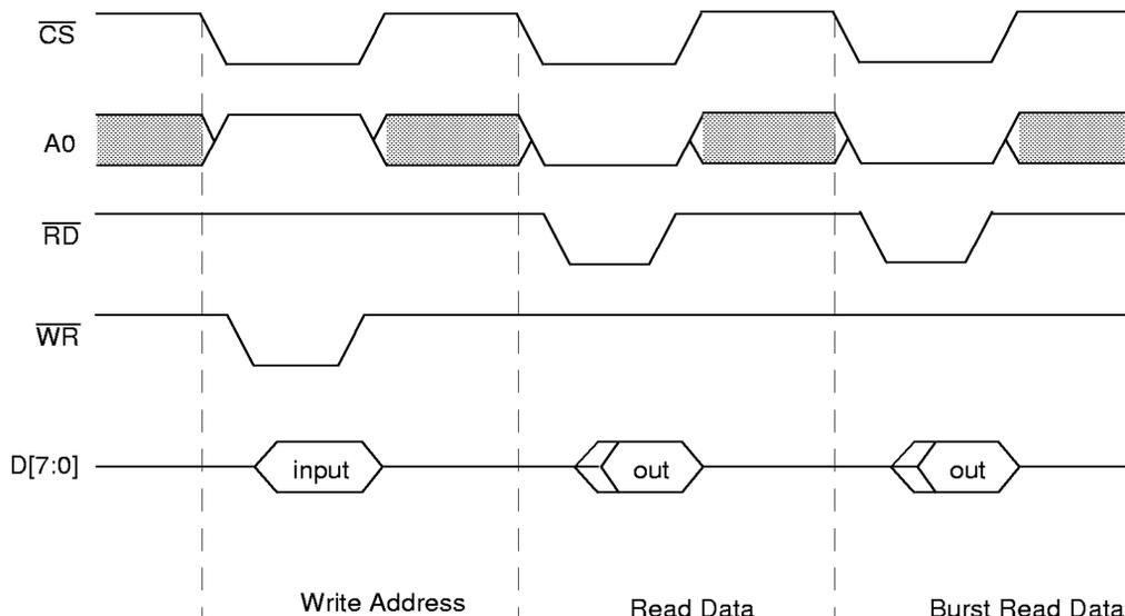
Figure 4. Non-Multiplexed Mode Basic Timing Diagram
