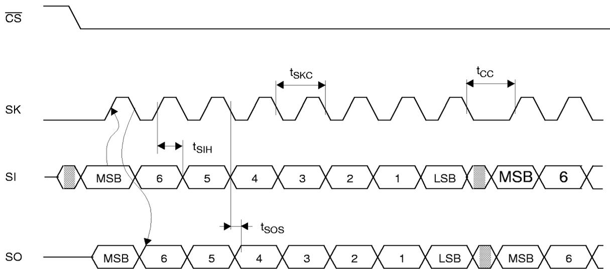
NOTE: The first eight SK cycles shift out the current contents of the shift register.
