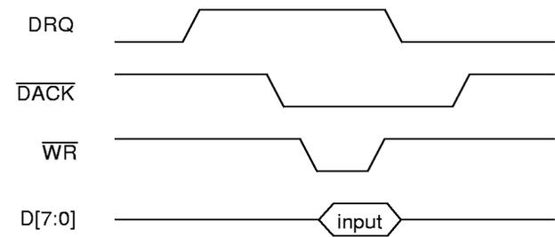
Figure 8. DMA Write to USBN9602
