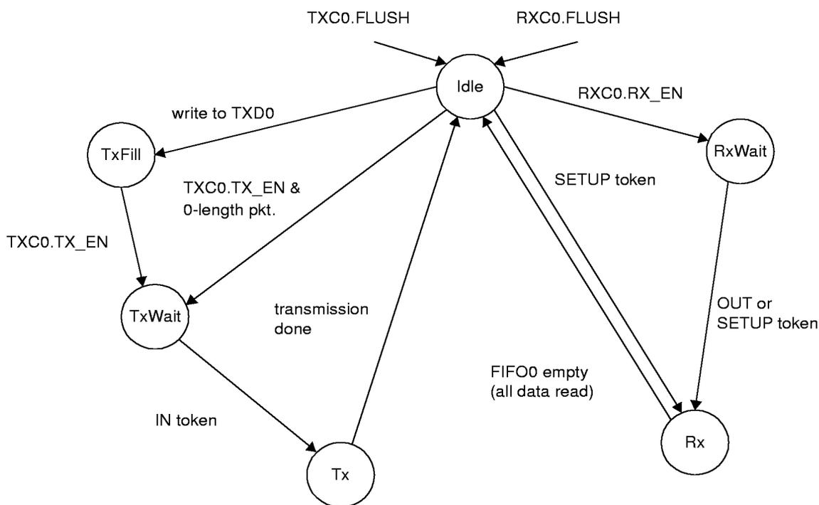
Figure 16. Endpoint 0 Operation
