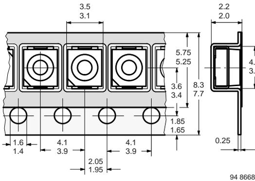
Figure 8. Tape Dimensions in mm for PLCC-2
