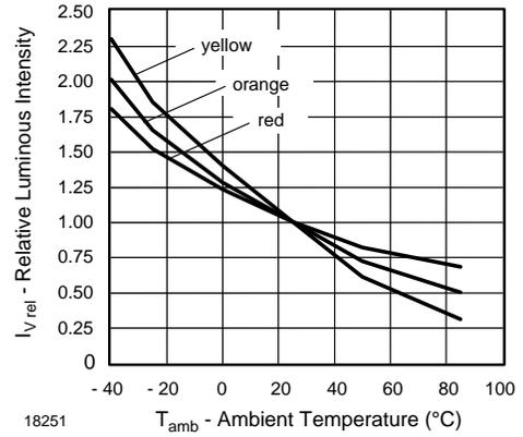
Figure 6. Rel. Luminous Intensity vs. Ambient Temperature
